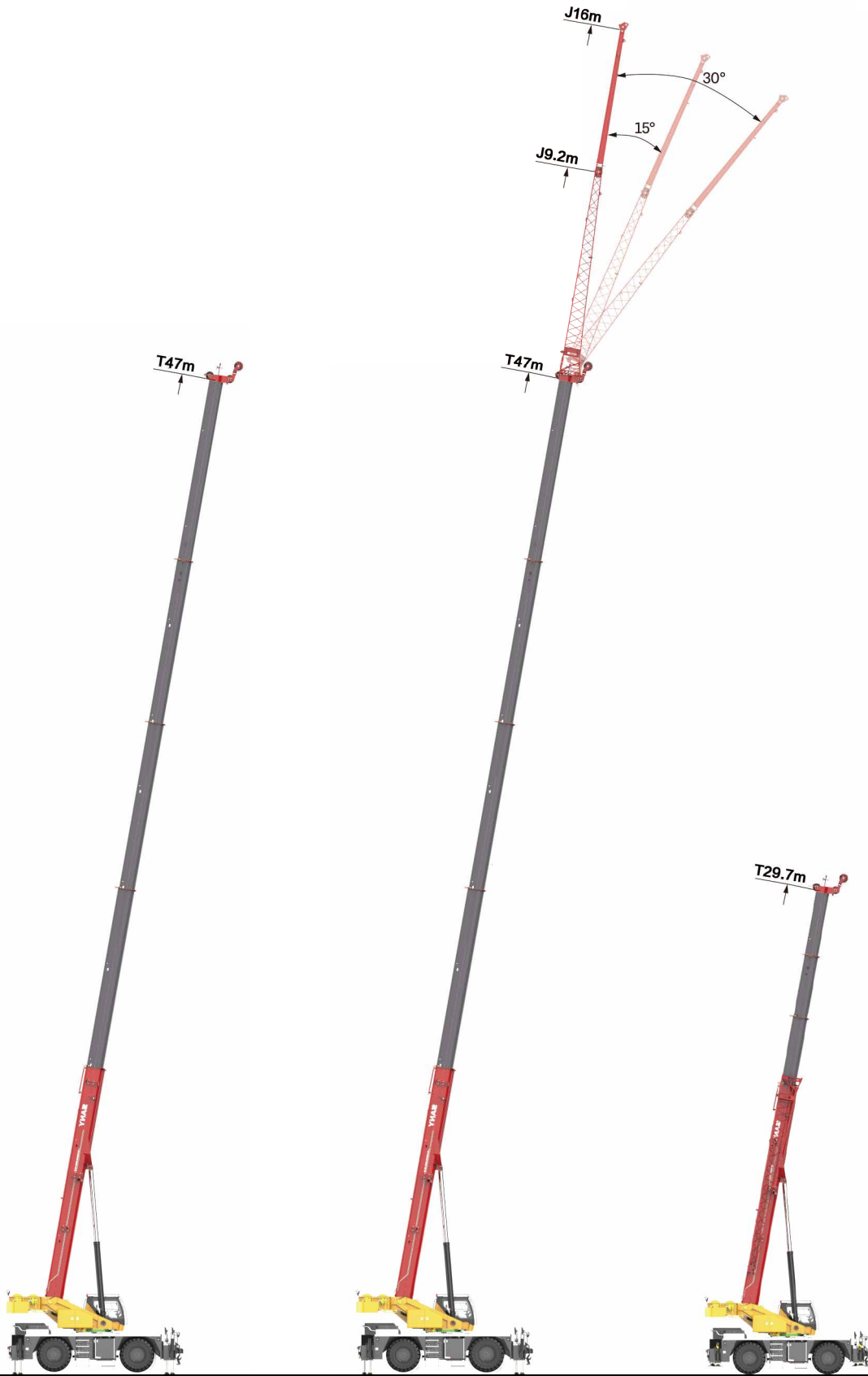
Telescopic boom on outriggers 主臂、支腿吊载
